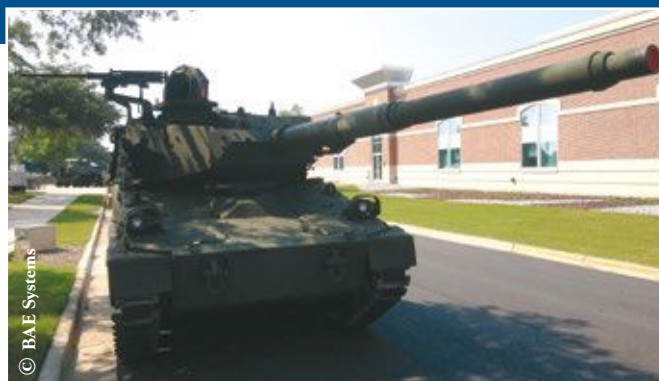
Equipped with a 105 mm main weapon, the M8 Armoured Gun System (AGS) can be described as a light tank, weighing up to 23 tons. Serial production of the M8 AGS, which was developed to replace the M551 Sheridan light tank, never began, as the US Army preferred the 8x8 Stryker vehicle family according to its new combat doctrine.
