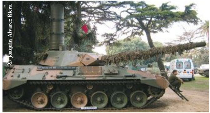
Developed to meet the requirements of the Argentinian Land Forces, the Tanque Argentino Mediano (TAM) medium tank is based on the German Marder armoured combat vehicle. Unlike Marder, this vehicle uses a turret equipped with a 105 mm main gun.
