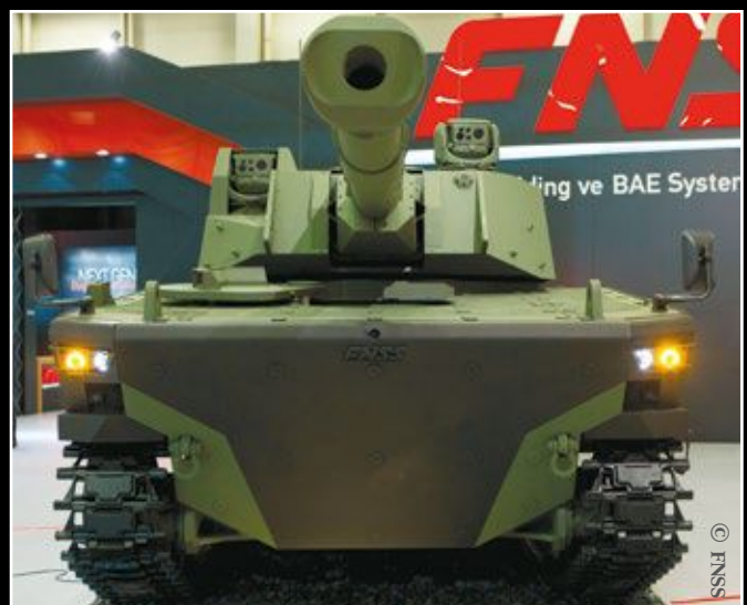
With a maximum weight of 35 tons, the KAPLAN MT has been developed to cross soft ground and bridges with a low load-bearing capacity, which tend to be highly inaccessible to main battle tanks.
