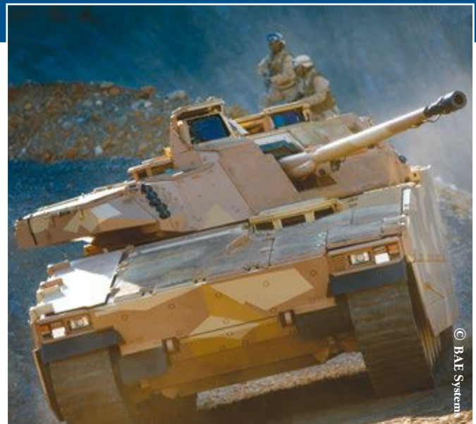
The CV90120-T light tank (left) has been developed on the CV90 platform that is also used for the CV9035 (right) armoured combat vehicle. Thus, a platform with a design weight of 20 to 25 tons was converted into a vehicle operating under a load ranging from 30 to 35 tons. The KAPLAN MT is a more coherent and balanced system within itself, having been designed as a tank from the very outset.
