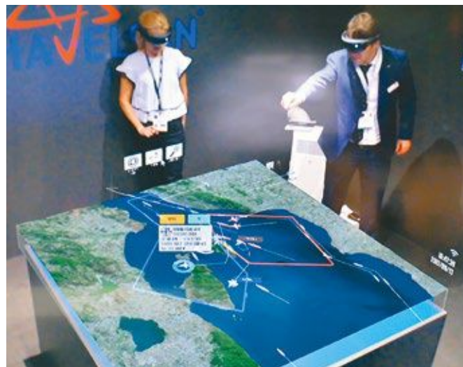
The HoSA-C4ISR displayed at the exhibition is essentially an augmented reality application for command and control purposes. Under the rapidly changing conditions of the battlefield, the HoSA-C4ISR enables, through its special glasses, the processing of large quantities of external data that would otherwise be difficult for humans to efficiently perceive and process, such that this data can be presented in a three-dimensional and visual format. When the special glasses of the system are not used, all that appears in an empty table (left). On the other hand, the screen outside containing the system shows the camera images of the room, overlaid with the images seen by the users wearing the special glasses. (right)
